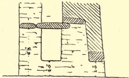
Figs. 164, 165.—Ground plan and section of elevation of doorway and passages through the wall of Broch in Glenbeg. (Drawn by J. Romilly Allen.)
